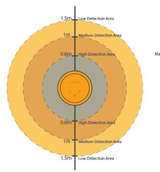
Varying magnetic field detection zones. The grey area depicts a 0.6m high sensitivity detection area surrounding the e-loop, suitable for the majority of vehicles. The dark colour area depicts a 1m medium sensitivity detection area surrounding the e-loop, suitable for most vehicles. The light colour depicts a 1.5m low sensitivity detection area surrounding the e-loop, which is only suitable for some vehicles. Radar Read Distances
