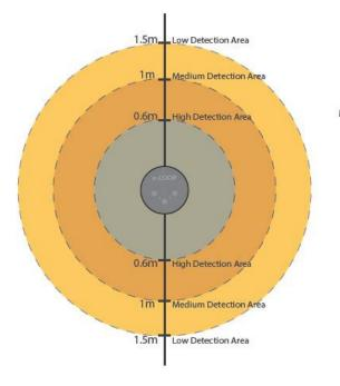
Varying magnetic field detection zones. The grey area depicts a 0.6m high sensitivity detection area surrounding the e-loop, suitable for the majority of vehicles. The dark colour area depicts a 1m medium sensitivity detection area surrounding the e-loop, suitable for most vehicles. The light colour area depicts a 1.5m low sensitivity detection area surrounding the e-loop, which is only suitable for some vehicles. Radar Read Distances
